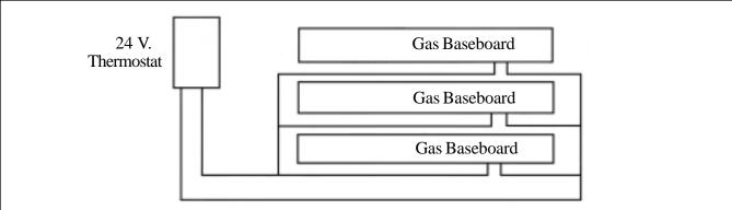
When wiring more than one baseboard heater to a single thermostat, the baseboard heaters must be wired in PARALLEL. When wiring more than one baseboard heater to a single 24 VAC thermostat, the baseboard heaters must be hard wired in parallel. Do not use cord sets. Do not cross thermostat connections between heaters. Purple thermostat connection from first heater to purple thermostat on second and third heater. Do the same with white thermostat connection.
